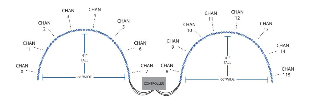
Plug each strand into its designated channel according to the diagram above.
