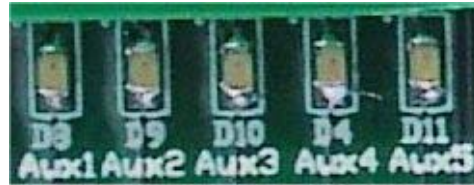
The Aux1 LED turns on when the controller is running in Smart mode. The other LEDs are reserved for future use.
