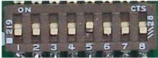
8-position dip switches for setting Dumb or Smart mode and for controlling channel outputs.
